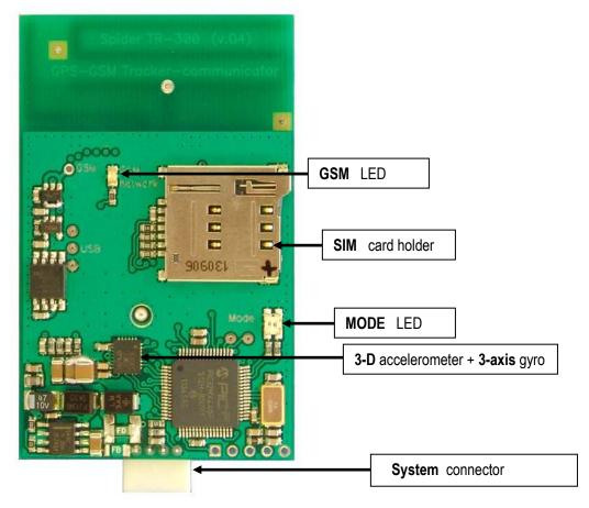
**GSM** LED **off** GSM-modem is off
